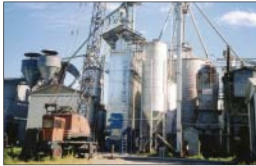
New Delux continuous-flow dryer at Louis J. Gale & Son Inc. in Waterville, NY, including an overhead protective covering. Photo courtesy of Louis J. Gale & Son Inc.
